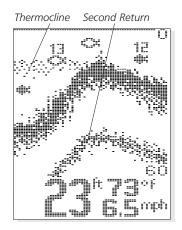
**Fish ID.** The Tracker unit uses advanced signal processing to further evaluate any sonar return between the surface and the bottom. For instance, a small school of bait fish usually appears as a dense cluster of individual dots. If the return meets certain additional criteria, a fish symbol will be assigned.
